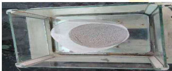
Plate 1: Grinded Periwinkle Shells Formulation of Water-Based Drilling Muds
