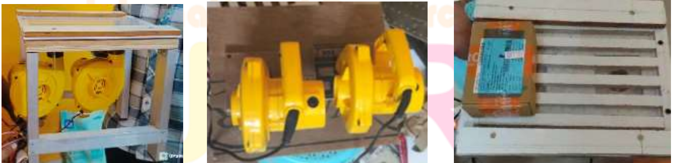
Fig: 5: Contactless Air Conveyor's Blower & with Conveying Product
