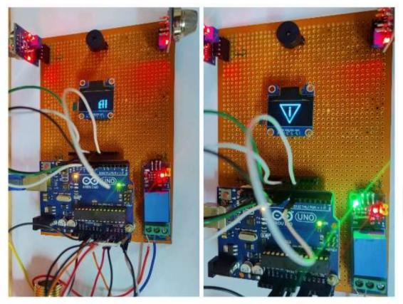
When the gas sensor is triggered, the buzzer activates, a caution symbol appears on the OLED display, and the relay is turned on.
