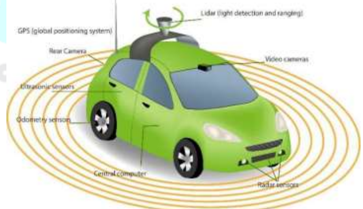
Fig-1.1: Autonomous car with camera, LiDAR, and radar sensors
