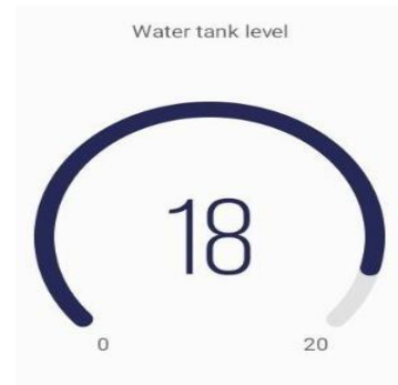
Fig 2: Water Tank level (Ultra sonic)
