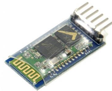
Figure 3(c): Bluetooth Module (HC-05)
