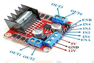
This high power motor driver module, the L298N, can drive stepper and DC motors. This module is made up of a 78M05 5V regulator and an L298 motor driver integrated circuit. The L298N Module may control two DC motors with directional and speed control, or up to four DC motors.
