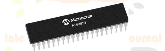
The AT89S52 is a CMOS 8-bit microcontroller that combines excellent performance and low power consumption. It has 8K bytes of internal programmable Flash memory. With the AT89S52, the following features come standard: Clock circuits, a full duplex serial port, 32 I/O lines, 8K Flash, 256 RAM bytes, three 16-bit timer/counters, a watchdog timer, two data pointers, a six-vector two-level interrupt architecture, and watchdog timers
