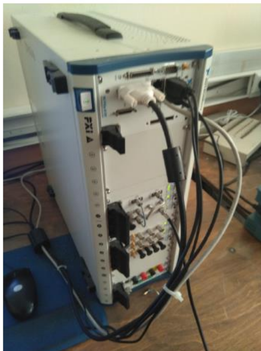
Fig. 2: The used digital oscilloscope type PXI-5114
