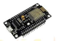
The ESP8266 is a key component enabling our smart notice board to connect to a Wi-Fi network and achieve remote communication. This highly-integrated chip from Espressif Systems offers a cost-effective and feature-rich solution for wireless connectivity in IoT projects. Here's a closer look at the factors that influenced our decision to utilize the ESP8266 in this project:
