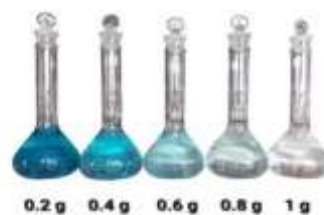
Figure 17. Adsorption of Methylene Blue dye using a sample of activated carbon - 5 th Day
