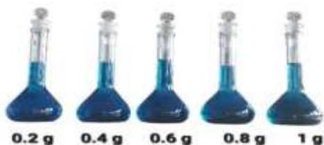
Figure 18. Adsorption of Malachite green dye using a sample of activated carbon – 1 st Day
