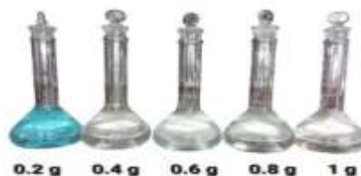
Figure 19. Adsorption of Malachite green dye using a sample of activated carbon - 5 th Day
