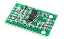
The HX711 module is a Load Cell Amplifier breakout board that allows you to easily read load cells to measure weight. This module uses 24 high-precision A/D converter chips HX711. It is specially designed for the high precision electronic scale design, with two analog input channels, the internal integration of 128 times the programmable gain amplifier.
