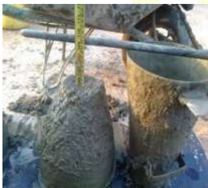
Fig 3.5 Slump Cone Test
