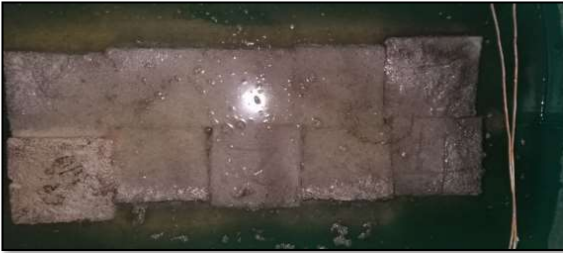
Fig 3.11 The exposure of cubes in H_2SO_4 solution.
