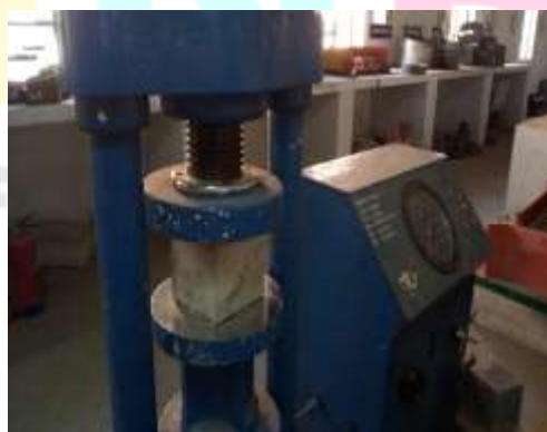
Fig 3.7 Compression Strength Test
