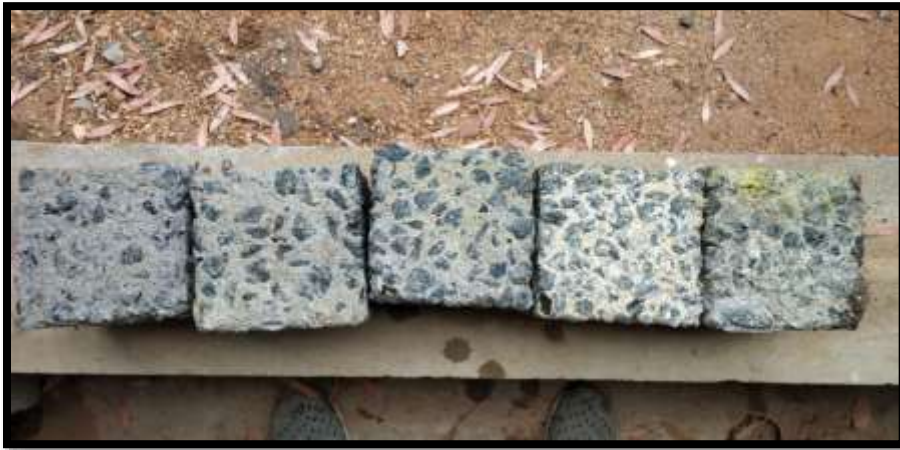
Fig 4.9 Cubes after exposure to H_2SO_4
