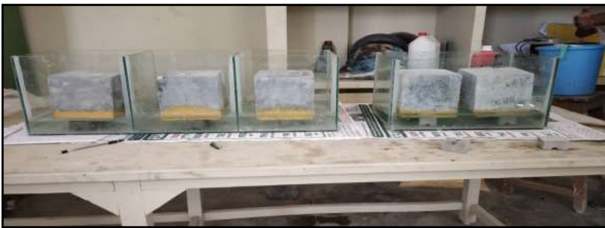
Fig 3.10 Sorptivity test setup
