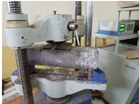
Fig 3.9 Flexural Strength Test
