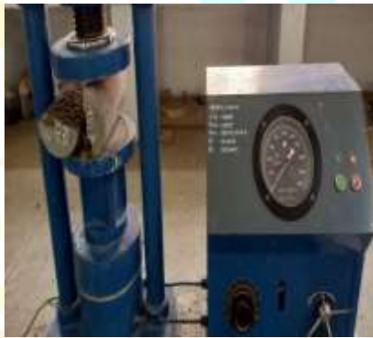
Fig 3.8 Split Tensile Strength Test
