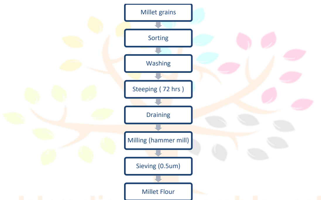
Fig.1. Flow sheet for making Millet Flour
