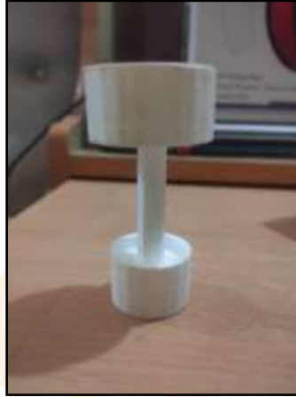
Fig.4.1: Double Headed Piston
