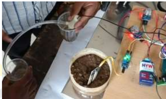
Fig 12: Working of Moisture sensor
