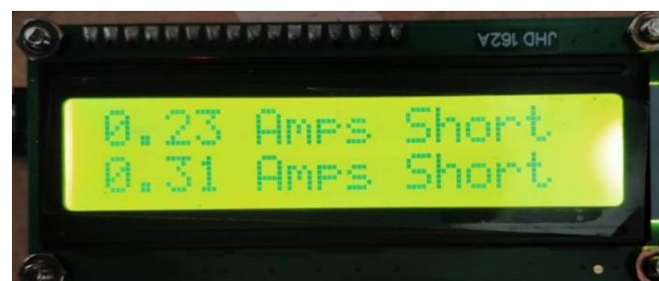
Figure:5 LCD Displaying L-L fault
