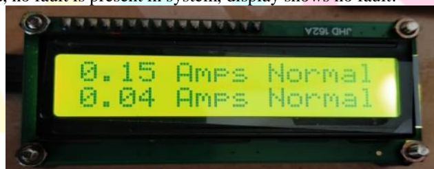
Figure:4 LCD Displaying normal (Without faults)
