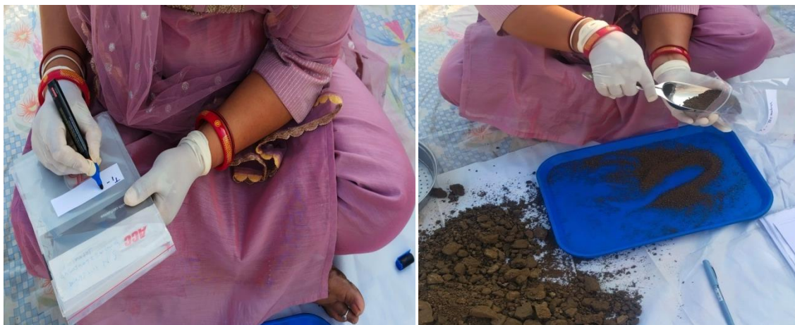
(Figure 5- Preparation of soil samples, Labeling of soil samples )
