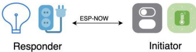
Fig 20: This shows how the ESP-Now works. The one which sends data(Sensor Node) is called the initiator and the one which receives is called the responder, the connection is full duplex.
