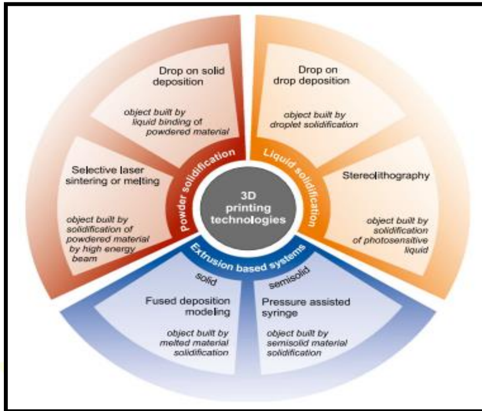
Fig. 4: 3D printing methods applied for drug formulation. [26,39]
