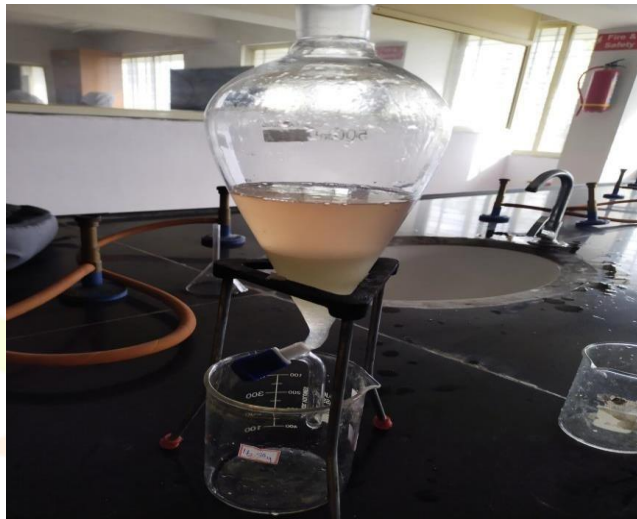
(Separate the chloroform and water with the help of separating funnel)
