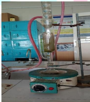
Fig 2: Soxhlet Extraction of Glochidion Zeylanicum
