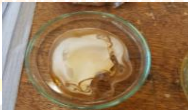
Fig. 2.3 Film preparation by casting
