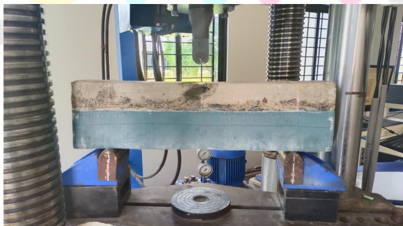
Fig 1: Vertical Grain Wrapped Beam
