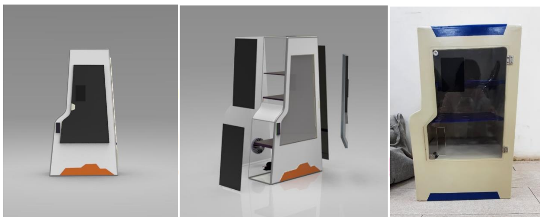
Figure 6: (from left to right) (a) 3D Model of Final Concept for Kiosk, (b) Exploded view of Kiosk, (c) Finished 1:3 prototype of Kiosk
