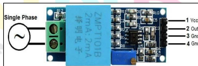
Figure 0-4:ZMPT101B AC voltage sensor module
