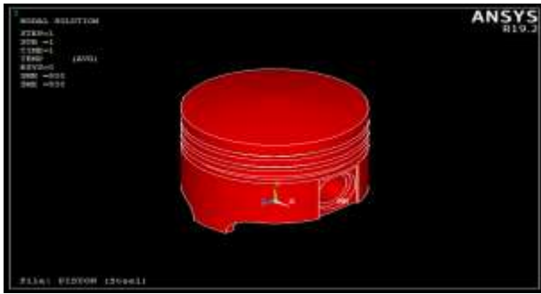
Fig. 7.11: Nodal Temperature of Piston – Forged Steel
