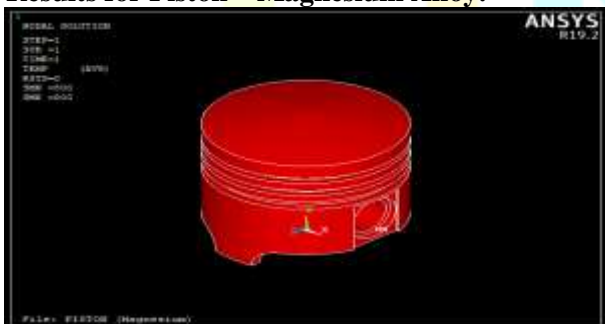
Fig. 7.6: Nodal Temperature of Piston – Magnesium Alloy
