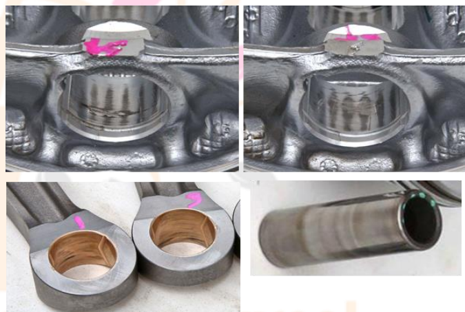
Figure 8: Piston, rod & pin post statistical clearance scuff test
