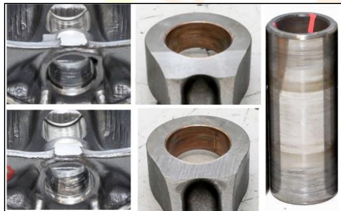
Figure 2: Piston, rod & pin post min clearance scuff test
