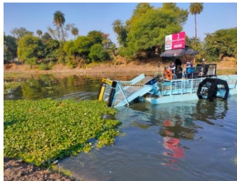
Fig5:- Using harvesters for collecting the aquatic weeds
