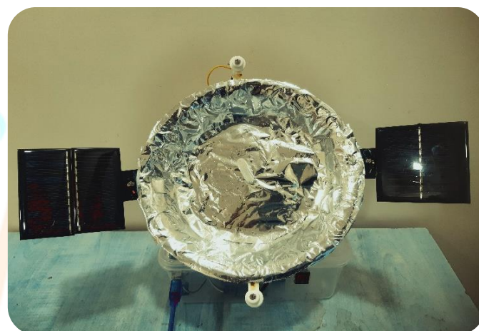
Fig 1: assembled solar dish system with dual-axis tracking
