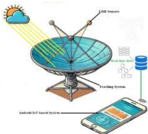
Fig 2: iot-based control flow for a solar dish
