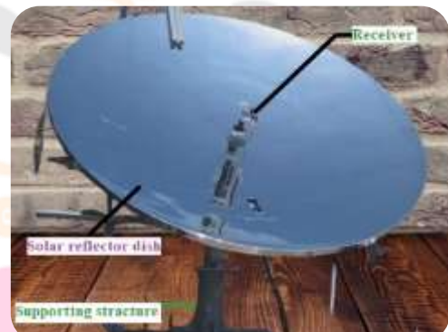
Fig 1: basic components of a solar dish system
