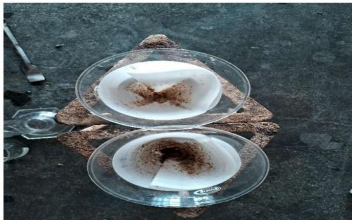
Figure 4. Filtration of the sulfur from ICS solution
