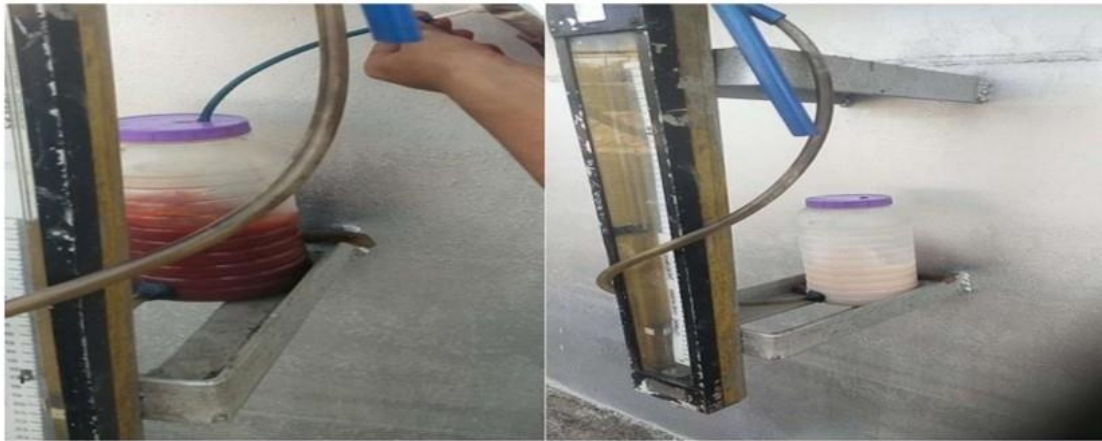
Figure 3. Colour change of the solution indicating formation of sulfur
