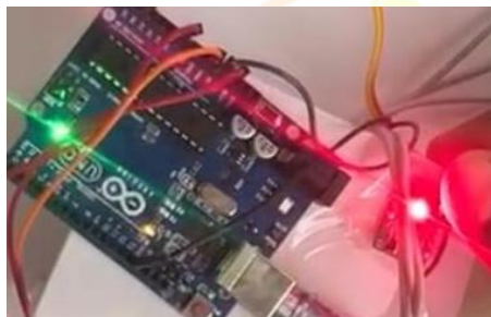
Figure 1. Arduino With Max30100
