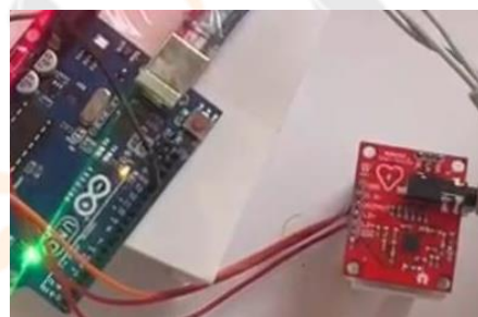
Figure 2. Arduino with AD8232 ECD Mod
