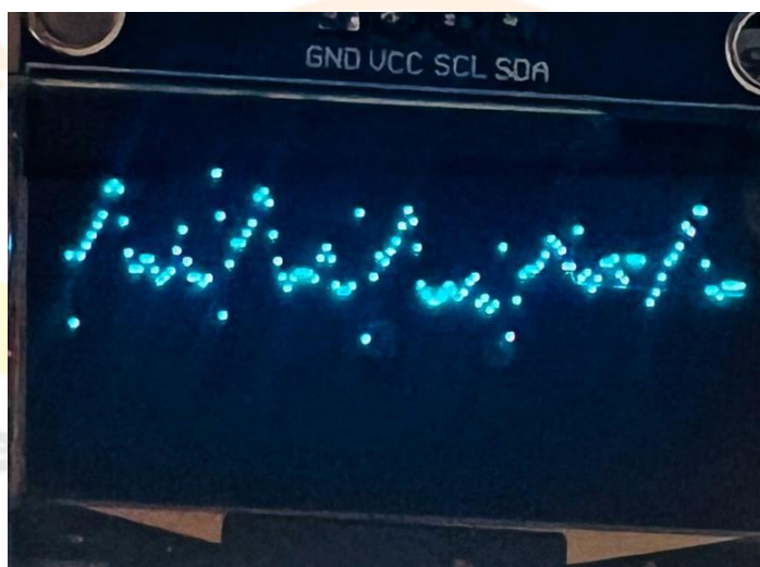
Figure 7. Output of ECG on 128 x 64 OLED DISPLAY
