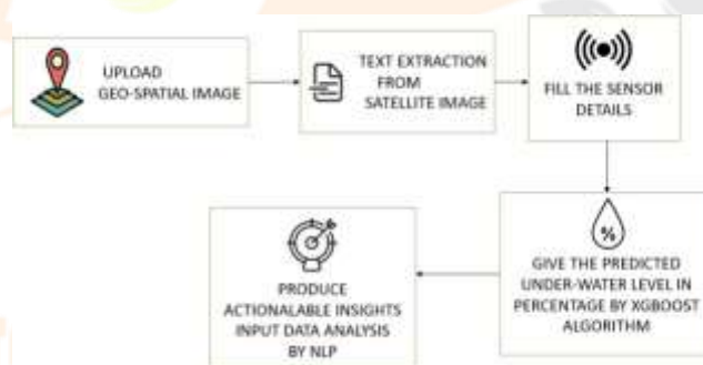
Fig.1.1. Under-Ground Water Prediction workflow
