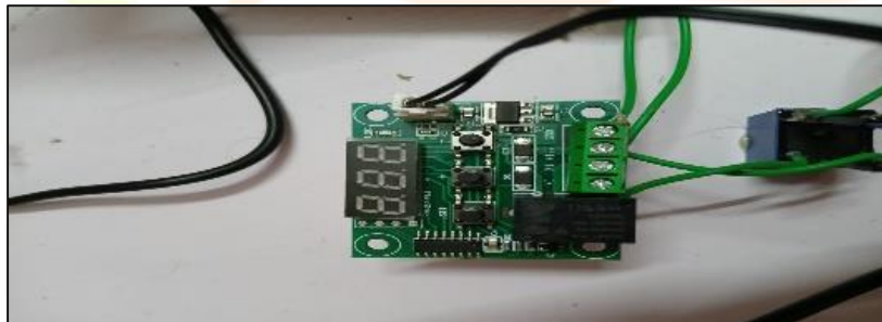
Fig. 4. (b) Over temperature detector
