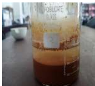
Fig 4.1.1 Sludge deposition and bubble formed after 2hrs incubation
