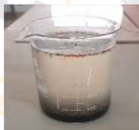
Fig 4.2.2 Sludge blanket formed after electrocoagulation
