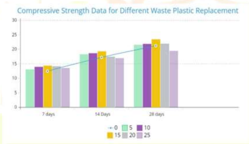
Figure 5.1: CS test results of M20 grade all concrete mixes
