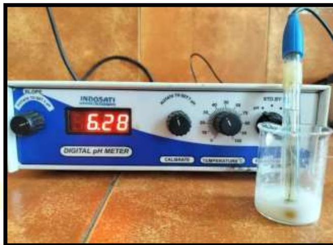
Fig.3 – pH test of lotion
