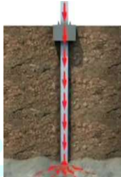
Fig 4: Pile foundation to transfer loads of steel frame structure though low soil bearing capacity of stiff soil with adequate bearing capacity
