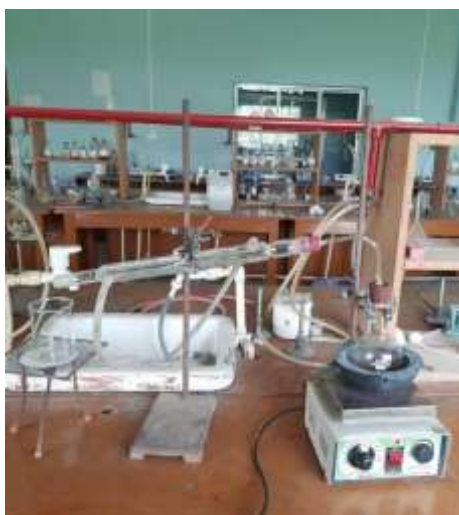
Steam distillation Setup
