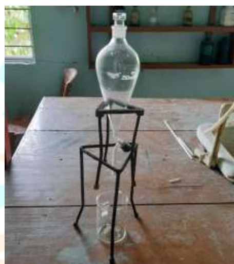
Separating Funnel Setup
