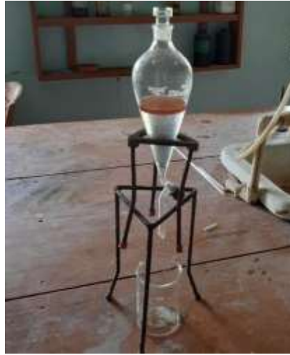
Funnel in two layer Oil is separated to the vial
