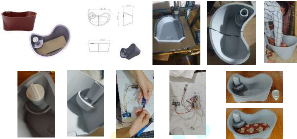
Figure 9: (from left to right) (a) Rendered Model of Final Concept, (b) Dimension drawing, (c) Prototype process (d) Finished 1:2 prototype of final concept
