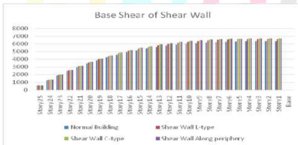
Fig. 5.3: Base Shear for Shear Wall System
