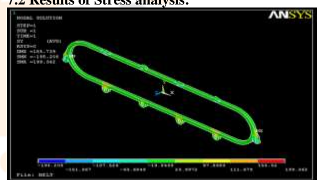
Fig. 7.2.1: Stress Analysis of BELT
