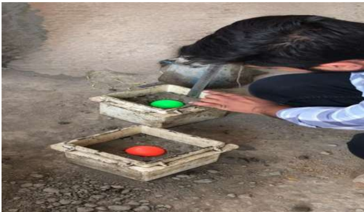
Fig.17 placing HDPE ball in cube
