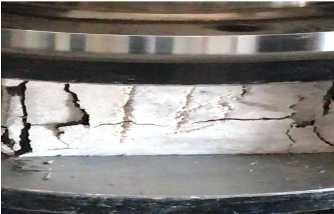
Fig.15 under compression testing machine
