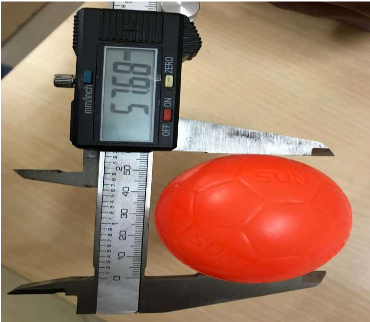
Fig.18 Taking diameter using vernier calliper
