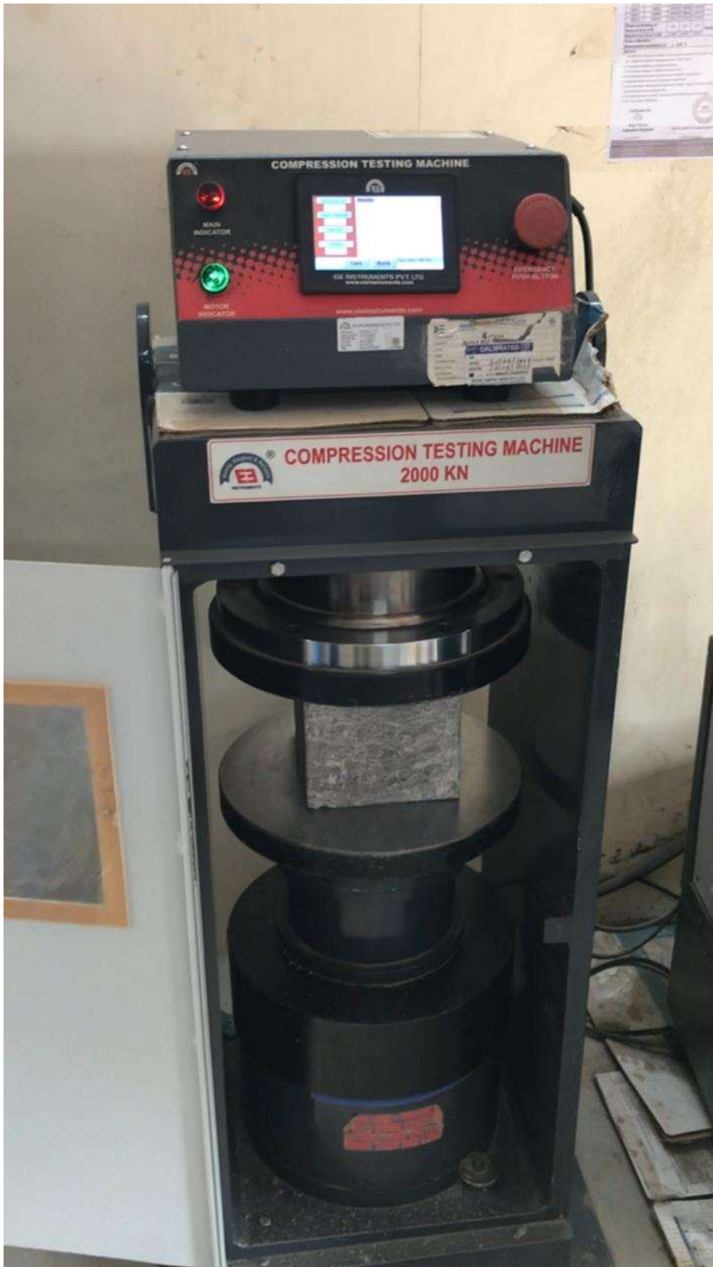
Fig.16 placing bubble deck cube in CTM
