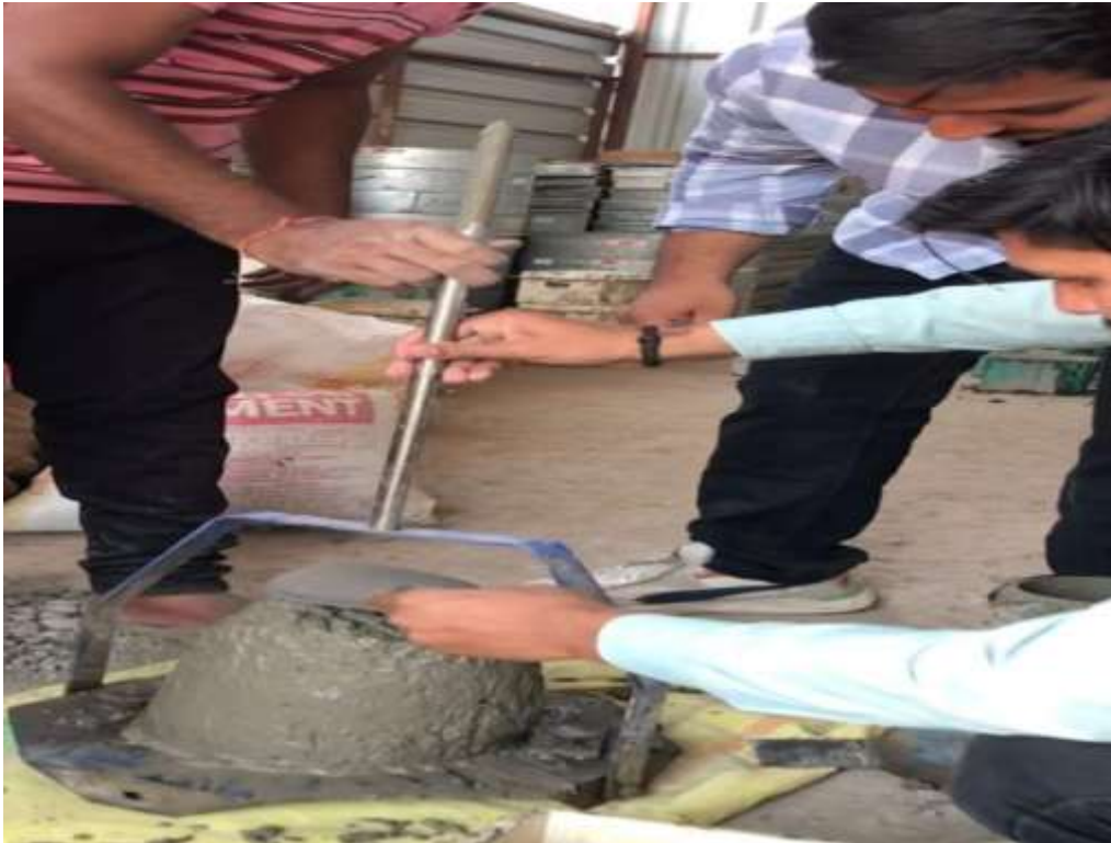
Fig.8 performing slump test
