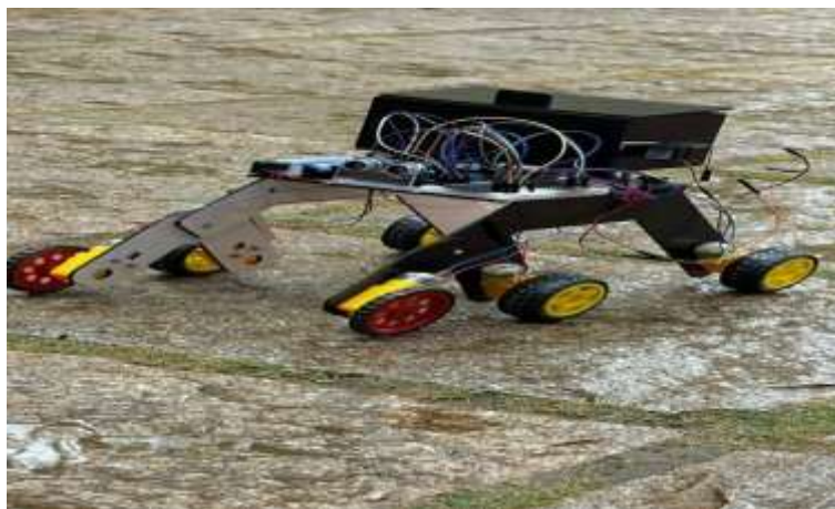
Fig. 2. Hardware prototype of the stair-climbing indoor delivery robot
