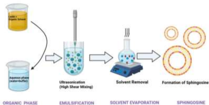
Figure 12: The image illustrates the solvent spherule method for the preparation sphingosomes using sphingolipid and cholesterol
