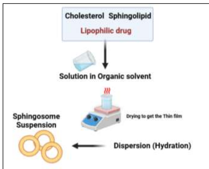
Figure 10: The image depicts the steps involved in the lipid film hydration method for the preparation of sphingosomes
