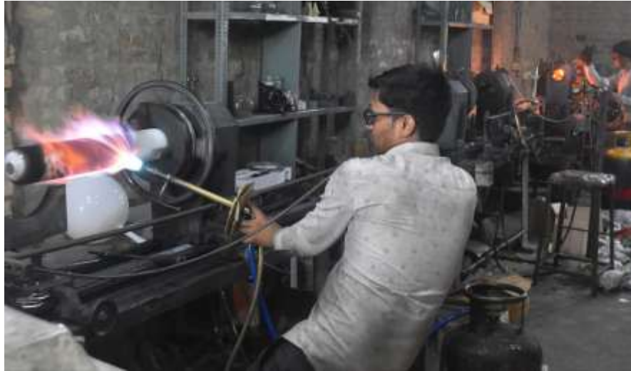
Figure 19: Artisan working with glass lathe machine
