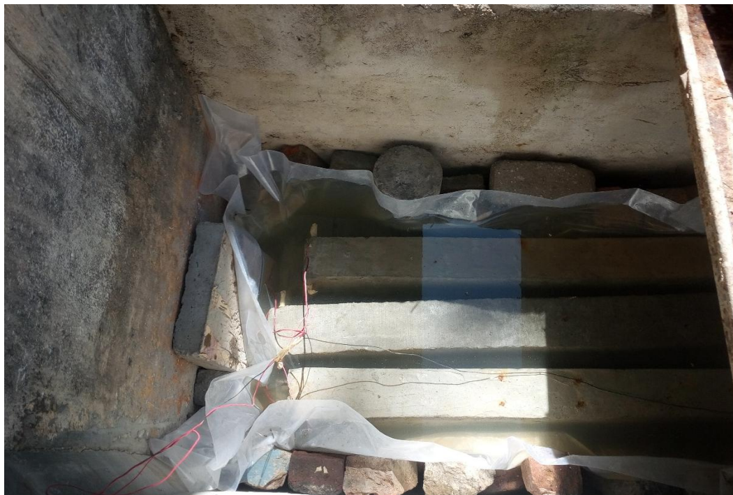
Figure; 5.8 Specimen partially immersion in 3% of NaCl
