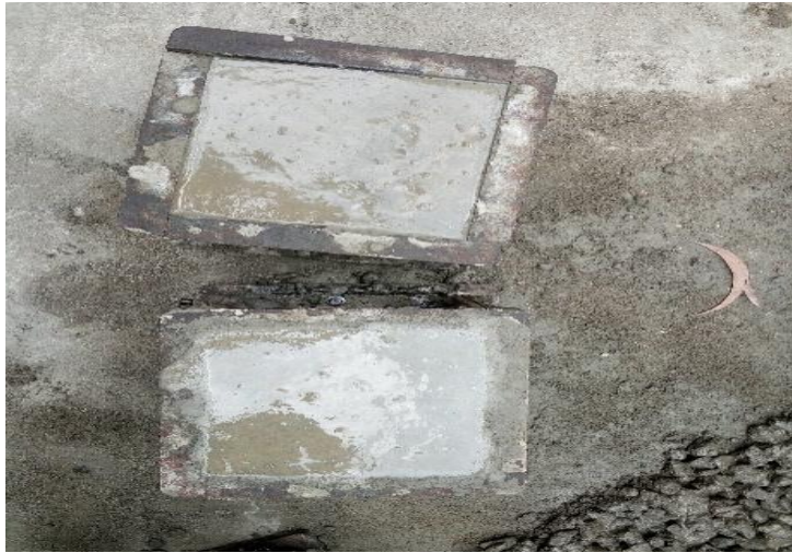
Figure 5.3 Casting of Cube
