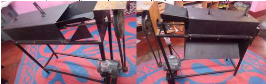
Fig. 4. Fabrication of portable corn deseeder
