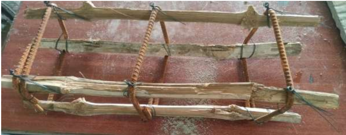
Fig: Bamboo Reinforcement
