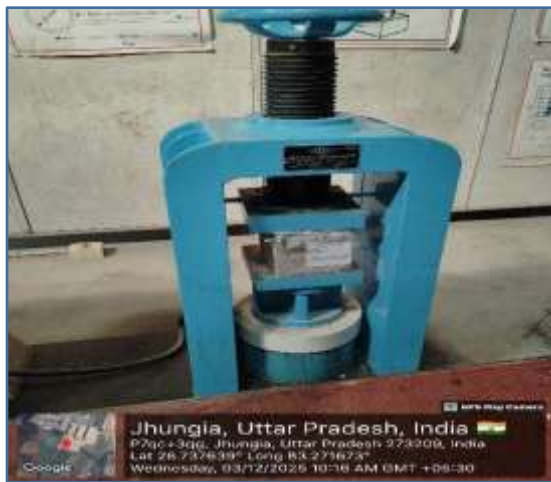
Fig:6 – Test In CTM Machine
